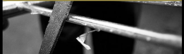
Dangerous edges are removed in the final stage of production by fettling. This gives a smooth and high quality finish.
