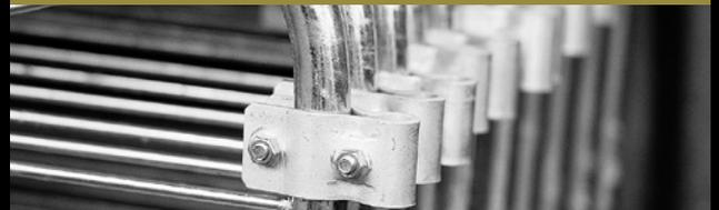
For improved strength and longer life, one piece adjustable clamps are added to the top and bottom of selected gates.
